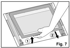
The internal pane of glass must be put back into the right seats as shown in Fig. 8.
